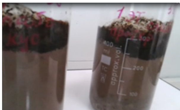
Figure 2- Oil release during heating of oiled soil
